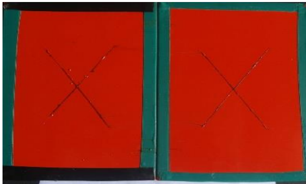
Salt Spray Test as a System on Phosphated Steel as per ASTM B-117 Test Method
