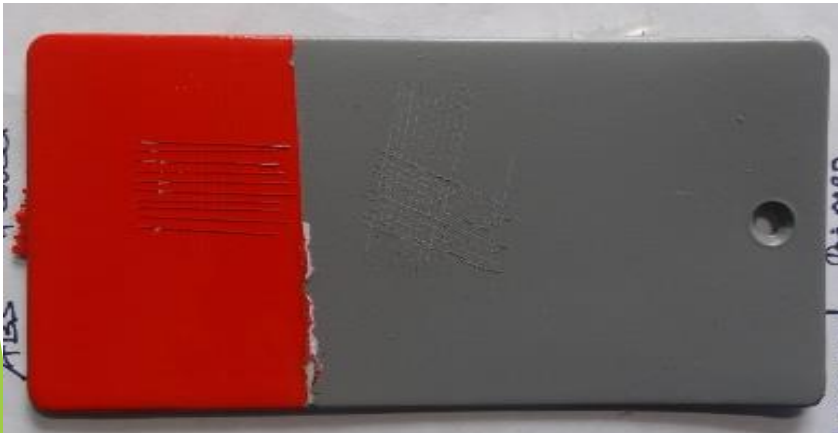
Salt Spray Test as a System on Phosphated Steel as per ASTM B-117 Test Method
