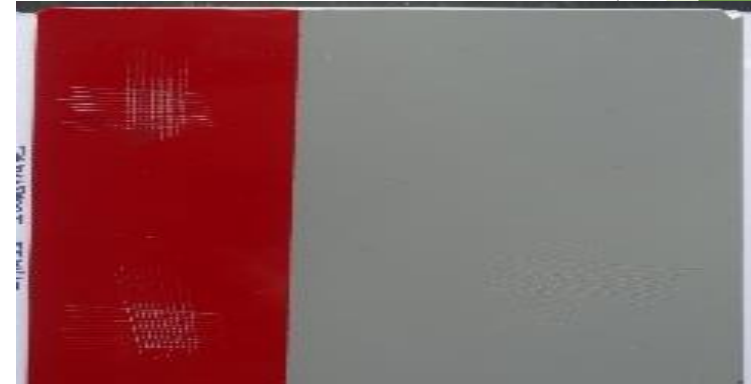
Adhesion Test on Glass as per ASTM D-3359 Test Method
