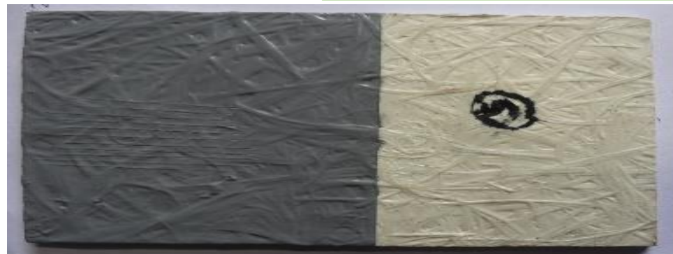
Adhesion Test on Glass as per ASTM D-3359 Test Method
